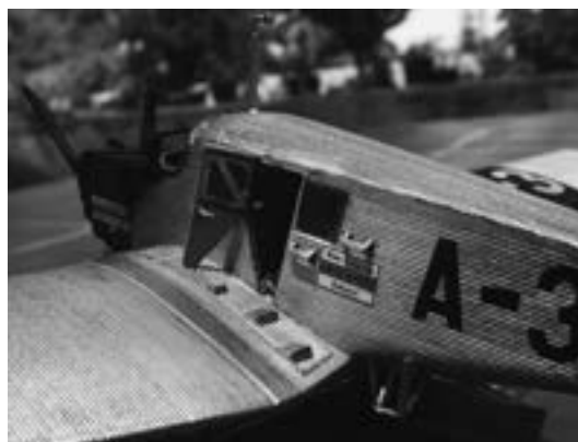
Fig. 11 Yunkers F.13 fabricated with corrugated panels of Duralmin sheets.
