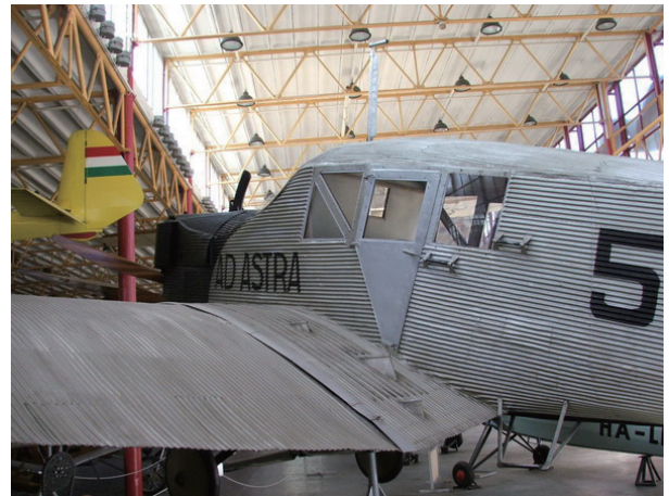
Fig. 8 All metal aircraft using corrugated duralumin sheet, Junkers F.13 (©2006 Andi Szekeres) 23) .
