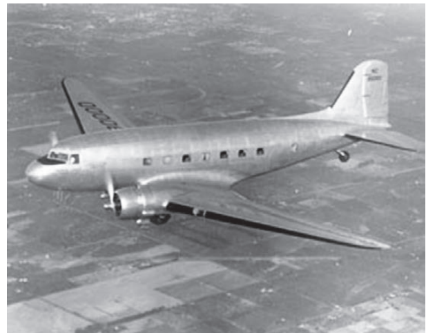
Fig. 7 DC-3 using Alcoa's Alclad 24S-T3 for the skin of the fuselage ( http://www.boeing.com/history/products/dc-3.page ).
