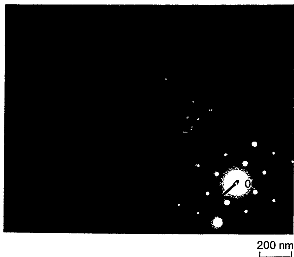
Fig. 10 Dark field TEM micrograph of \delta precipitates in an Al-2.5%Li binary alloy, solutionized and held at 573K for 10 3 s followed by water-quenched.
